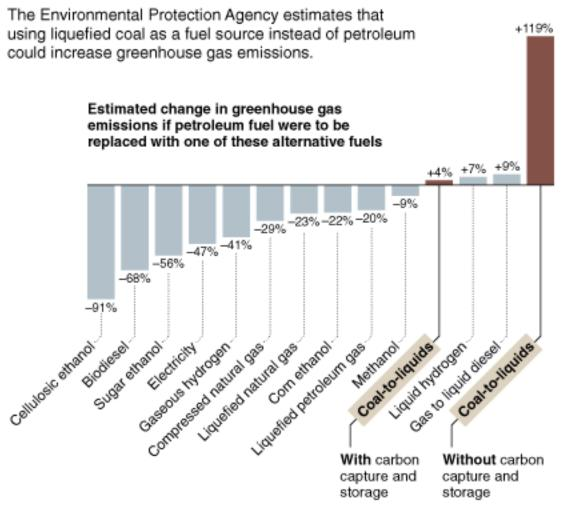
Note: The estimates include emissions from all parts of the process of making the fuels including fossil extraction, feedstock growth and distribution as well as averaging for the different methods of producing the fuels.
